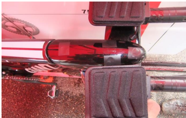
Figure 45: Illustration of the addition of tape to cover bolt access holes
