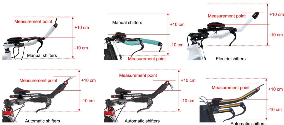
Figure 40: Points of measurement for the vertical limits of the handlebars extensions and any accessories
